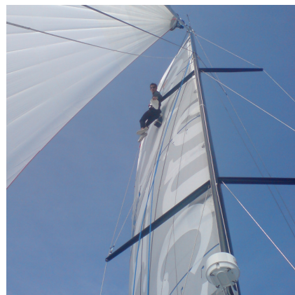
Fitting new spreader patches
